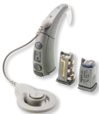
Nucleus® Freedom™ BTE with 3 zinc air batteries and rechargeable battery.
